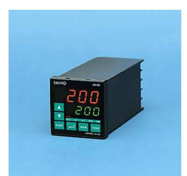
The model AK48 is a 48x48mm process controller with advanced featu-
